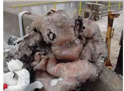
Photo 2: Combustible solid removed from the tank.
