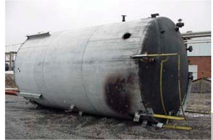
Photo 1 (above): Atmospheric storage tank following the fire.
