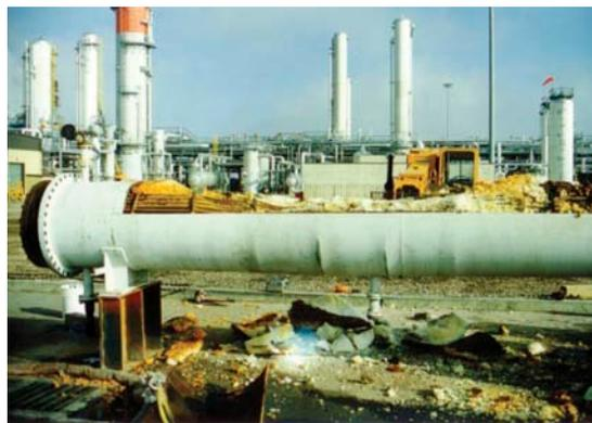
Photo 6: Deformed condenser shell.
